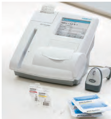
HbA1c (1 µL blood sample) and ACR (40 µL urine sample) results in 6 and 7 minutes.
